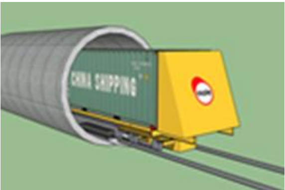
Shipping containers 4.5m dia 40ft, 30 Tonne
