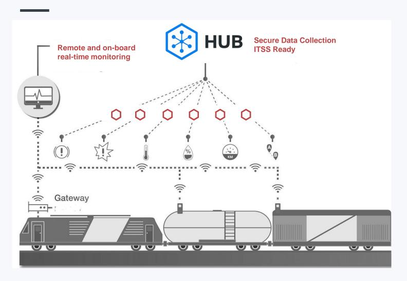
Extended reach capacity on board trains allows messaging via GSM
