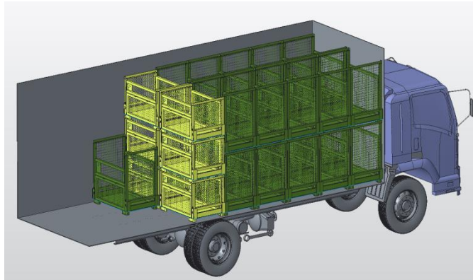
Figure 10. Improved stackability of foldable PI grid boxes
