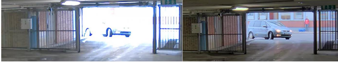
Figure 9: Difference between a non WDR (left) and a WDR camera (right)
